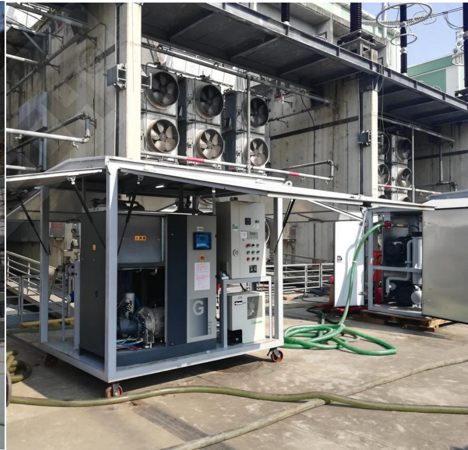
FUOOTECH Transformer Drying Air Generator for transformer maintenance
